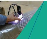
IIA's proprietary ARMUT<sup>®</sup> technology is the only system that combines automated and manual UT examination methods and uses a QR code film on complex geometry to gather encoded positional and encoded time data simultaneously. The ARMUT<sup>®</sup> can be used by a single technician to examine critical welds and gather extremely high-resolution images that can be stored, shared, and immediately analyzed.
