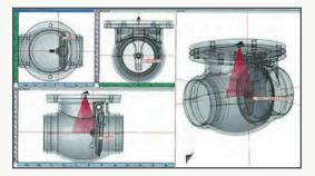
Industrial Inspection & Analysis Nuclear Services' division provides inspection and diagnostics services for a variety of valve configurations using our Phased Array Sectorial Scanning (PASS®) technique. In addition, our PASS® Visualization Software provides a comprehensive solution for Phased Array UT (PAUT) data analysis and field interpretation.
