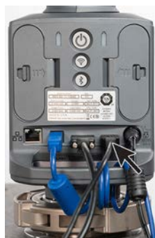
Figure 7-7 Connect the 8-Axis USB Cable
