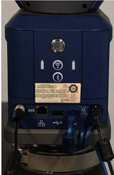
Figure 7-5 Connect the 8-Axis Cable
