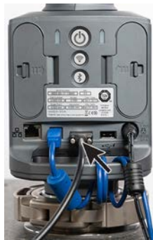
Figure 7-6 Connect the 8-Axis Cable
