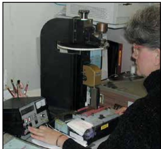
Gage Block Calibration at Starrett-Webber in Cleveland, Ohio
