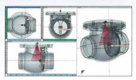
Industrial Inspection & Analysis Nuclear Services' division provides inspection and diagnostics services for a variety of valve configurations using our Phased Array Sectorial Scanning (PASS®) technique. In addition, our PASS® Visualization Software provides a comprehensive solution for Phased Array UT (PAUT) data analysis and field interpretation.
