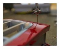
Need accurate data on small parts? A coordinate measuring machine (CMM) dimensional inspection is your best bet. But if you need to reverse engineer a part, a laser scan is a better choice.
