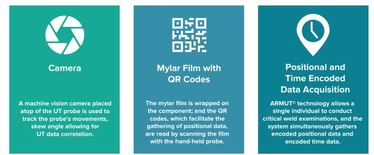
IIA's proprietary ARMUT<sup>®</sup> technology is the only system that combines automated and manual UT examination methods and uses a QR code film on complex geometry to gather encoded positional and encoded time data simultaneously. The ARMUT<sup>®</sup> can be used by a single technician to examine critical welds and gather extremely high-resolution images that can be stored, shared, and immediately analyzed.
